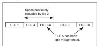
It is very important to avoid this type of fragmentation when recording sound files, as data quantities tend to be very large. If the disk drive must constantly jump around to look for free sectors, it may become unable to keep up with the incoming data. In the worst case, the recording will simply stop.
