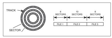
As files are deleted and new files saved, the disk can become cluttered with a random pattern of free and used spaces. A file that is recorded to such a disk tends to get split up over different areas, rather than stored on a contiguous series of sectors. The drive will have to jump all over the disk when reading or writing the data, resulting in a drop in the access speed.
