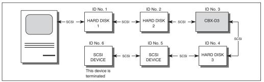
The example above shows seven devices (computer and six peripherals) connected in a SCSI daisy chain. Each device has a different ID number. Note that the last device in the chain is terminated. In most cases SCSI ID 7 is reserved for use by the computer, and ID 0 for the internal hard disk. Do not use either of these IDs for any other SCSI device.
