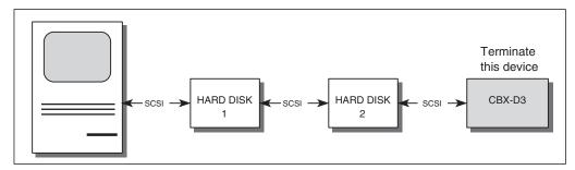
Some SCSI devices have a built-in terminator, and must therefore be connected at the end of the daisy chain. The CBX-D3 and many other devices utilize a detachable in-line terminator, as illustrated below.
