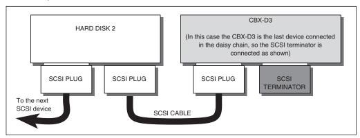
NOTE: If the SCSI daisy chain is not terminated correctly, numerous problems including data corruption, system crashes, and intermittent glitches can occur. If you have just set up your SCSI daisy chain or have added a new SCSI device to it and it is not working as it should, check that the SCSI daisy chain is terminated correctly. If the problem persists, try connecting the SCSI devices in a different order.
