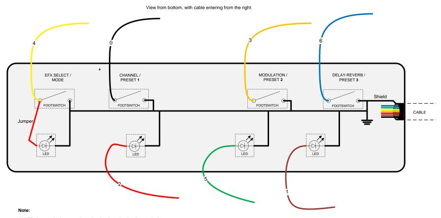
All LEDs have red wire to anode, spliced to the color the diagram indicates.
